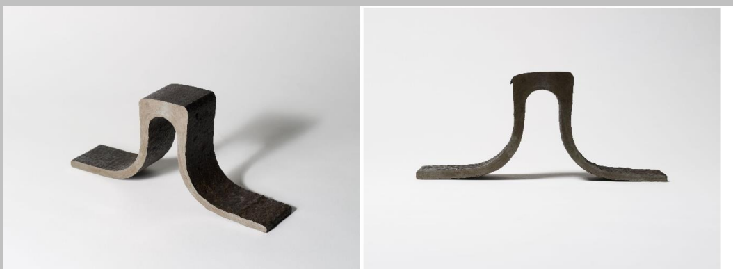
▲ B2446 Barlow rail, sections (3), wrought iron, used on first railway line between Sydney and Parramatta 1855-1877, made by Cruttwell, Allies & Co., Wales, 1854 Museum of Applied Arts and Sciences Museum of Applied Arts and Sciences
